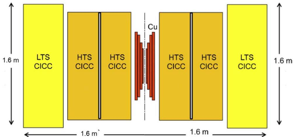
**Figure 3.** Preliminary concept design for a 60 T 'tri-brid' magnet. The copper Bitter magnet coils at the centre are surrounded by high-temperature superconducting cable-in-conduit conductors (HTS-CICC) that are in turn surrounded by a low- $T_c$  superconducting outsert [M. Bird, *IEEE transactions on Applied Superconductivity* 25, (2015)].
