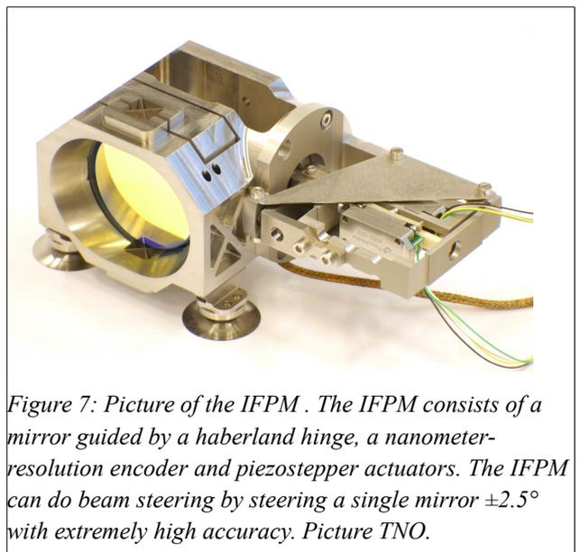
Figure 7: Picture of the IFPM . The IFPM consists of a mirror guided by a haberland hinge, a nanometer-resolution encoder and piezostepper actuators. The IFPM can do beam steering by steering a single mirror  $\pm 2.5^\circ$  with extremely high accuracy. Picture TNO.
