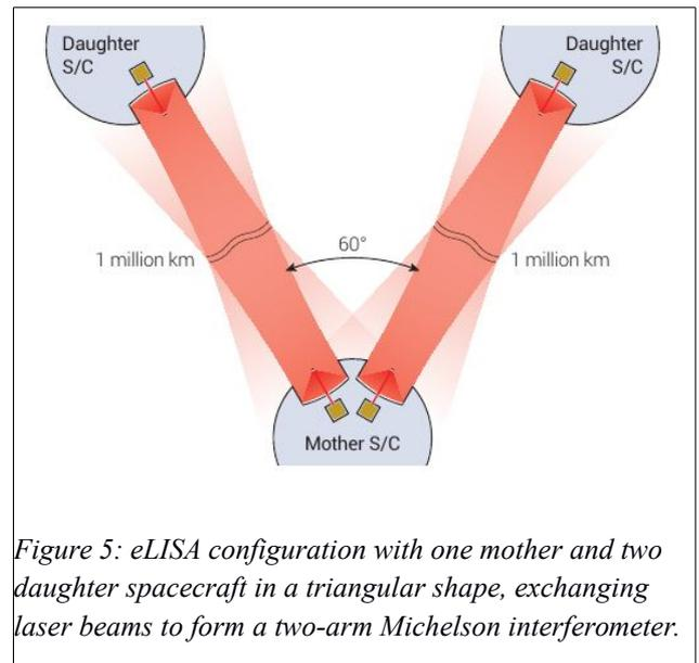
Figure 5: eLISA configuration with one mother and two daughter spacecraft in a triangular shape, exchanging laser beams to form a two-arm Michelson interferometer.
